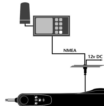
Fig 5.6 - Interfacing to Tillerpilot via NMEA
