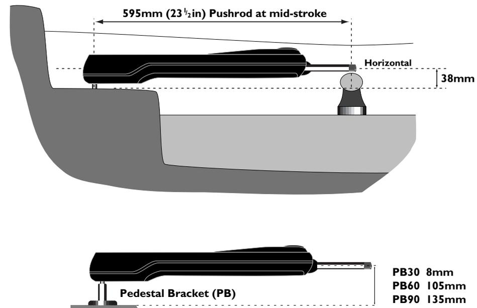
Fig 5.2 - Installation, cross section
