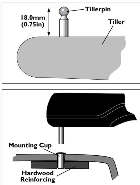
Fig 5.1 - Tillerpin & mounting cup
