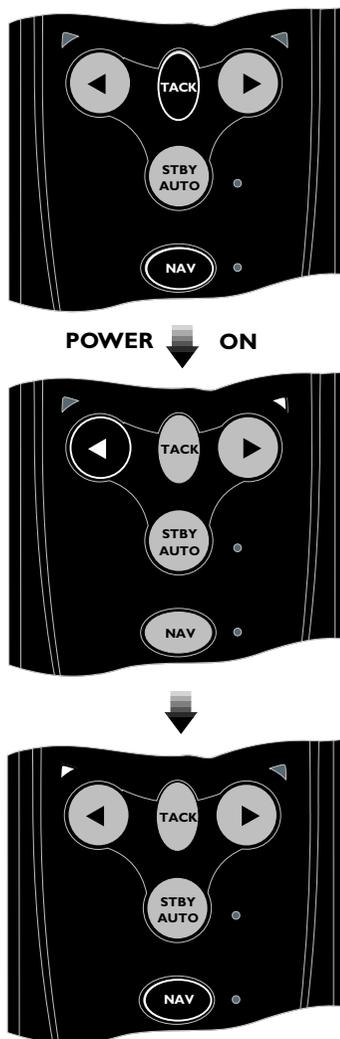
Fig 4.2 - Configuring for Port mounting
