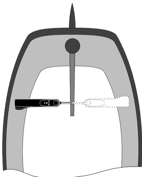
Fig 4.1 - Starboard and Port mounting options
