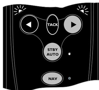
Fig 3.4 - Initiating Port Autotack in Sail To Wind Mode
