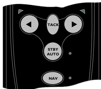
Fig 2.1 - Tillerpilot keypad
