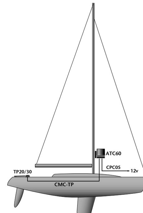
Fig 3.5 - Using TP20 / TP30 with external compass
