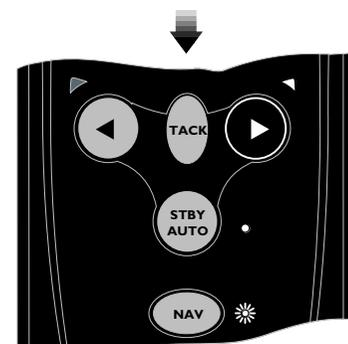
Fig 4.5 - Increasing Gain level
