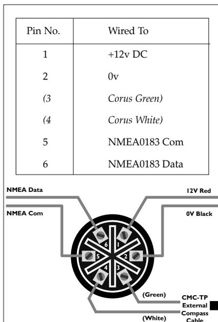
Fig 5.4 - Six pin socket connections - rear view
